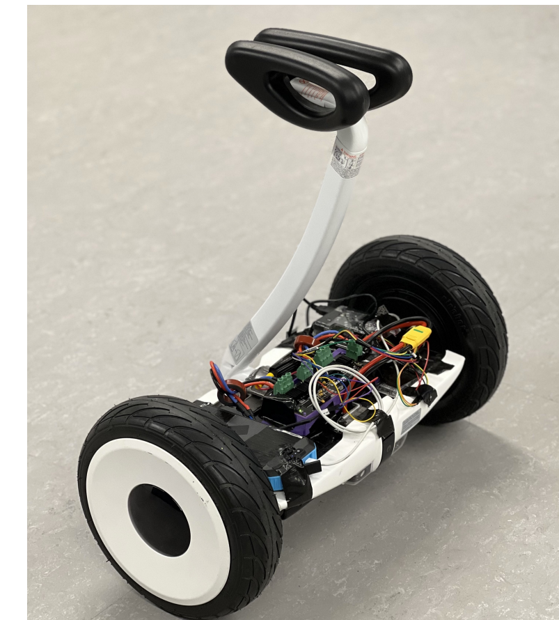
Figure 3: Modified Segway stabilizing autonomously
